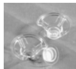
Snapwell inserts for use in diffusion or Ussing chambers
