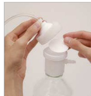
Place membrane filter on top of grid.
