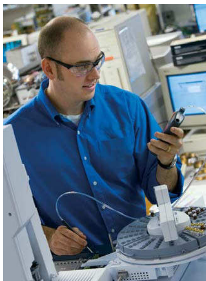
Scott Grossman, Applications Chemist Checking for leaks, using a thermal conductivity leak detector.
