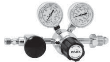
Inlet gauge: 0 to 4,000 psig (0–27,579 kPa) Outlet assembly: diaphragm valve, 1/4" tube fitting
