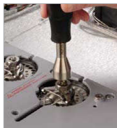
Slip tool over septum nut...
