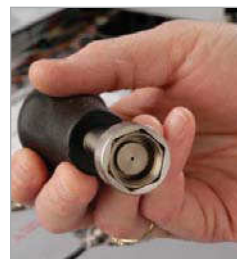
Septum nut remains in tool until reinstalled.
