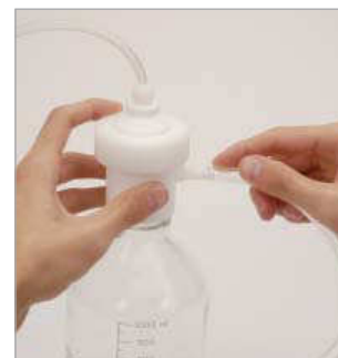
Connect vacuum line to side port.
