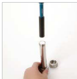
Place a filter at the top of the extraction cell.
