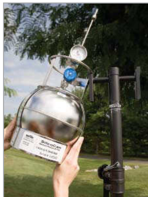
Air canister tripod conveniently holds two air canisters.
