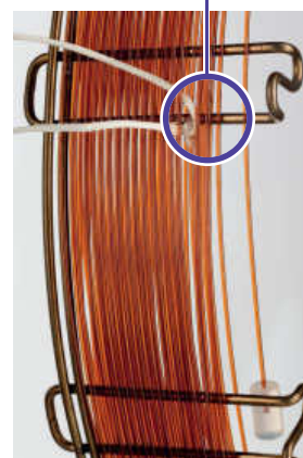
String indicates where the analytical column begins.
