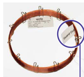
Tag indicates guard column end.
