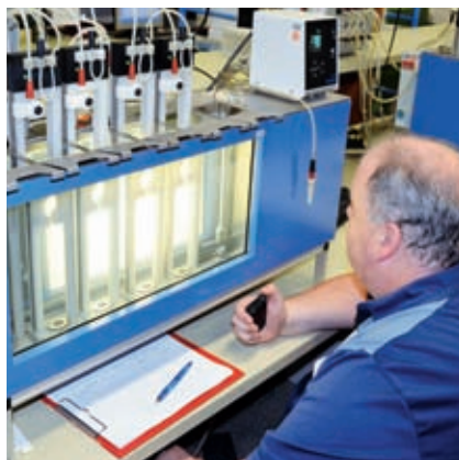
With the processed calibration, the viscometers are provided with an ID number and a certificate documenting the specific characteristics.
